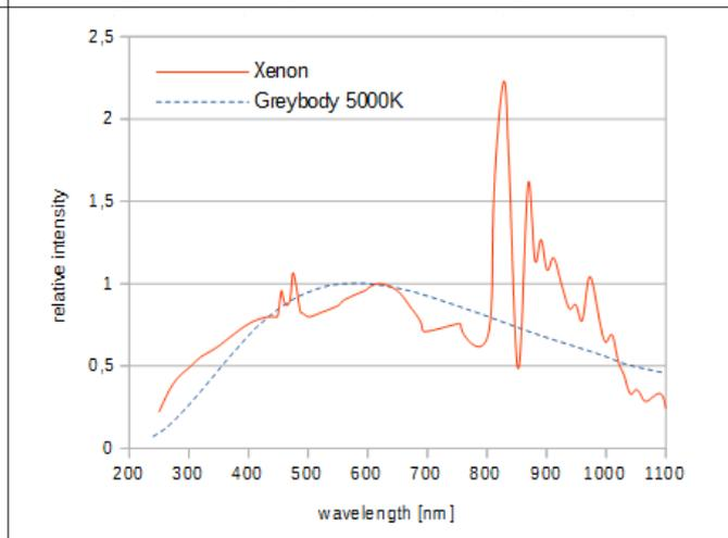
Fig.4. Relative spectrum of XEN light source
