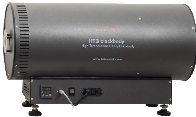
Fig. 1. Photo of the HTB-35D-1200 blackbody
