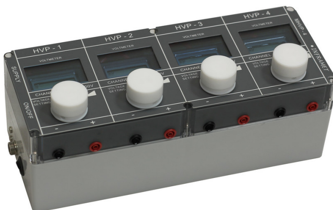
Fig. 1. Photo of HVP power supply
