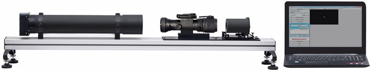
Fig. 2. Photo of NCLIP test station
