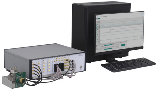
Fig. 1. CONIR universal system for control of IR FPA sensors
