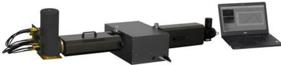
Fig. 5. FAPA-S system for spectral tests of IR FPAs/camera cores
