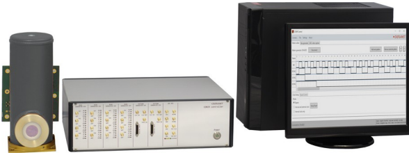
Fig. 1. CONIR universal controller for control of IR FPA sensors
