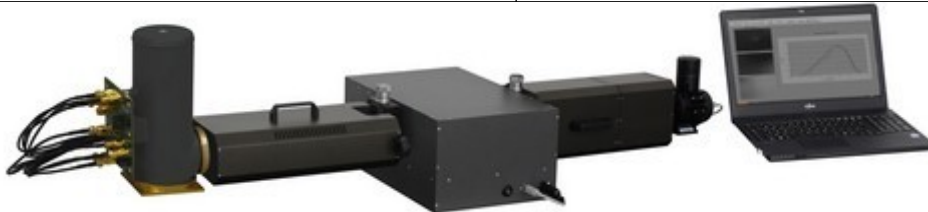
Fig. 5. FAPA-S system for spectral tests of IR FPAs/camera cores
