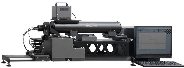
Fig. 3. FAPA-I system for image quality tests of IR FPAs/camera cores
