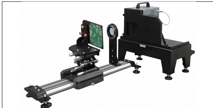
Fig. 1. FT-N configuration of FT test system (measurement of noise/responsivity parameters in static flood mode)
