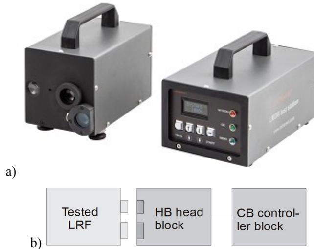
Fig. 1. LMOB test system: a) photo, b) block diagram
