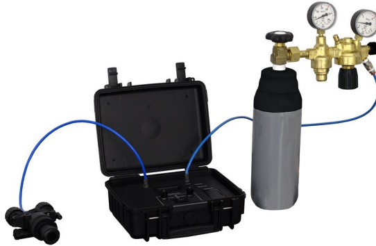
Fig. 1. Photo of the NPL purge-leak station
