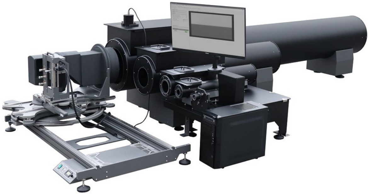
Fig. 1. Photo of ORIFA test station (MWIR/LWIR configuration)
