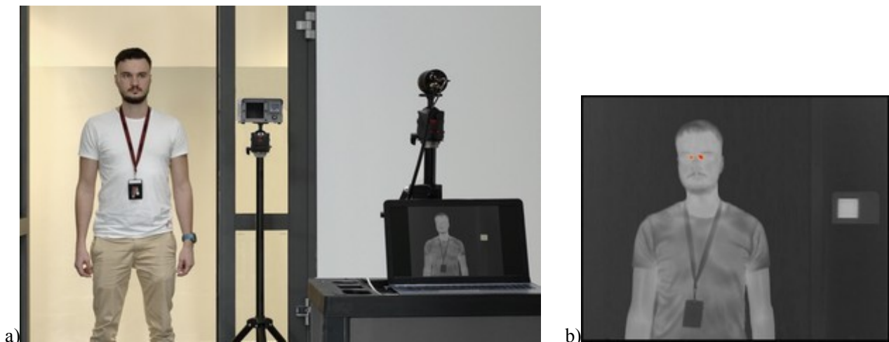
Fig.1. TREEN a)photo of thermograph system, b)thermal image of tested human
