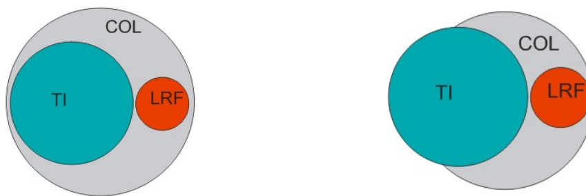
Fig. 4. Position of optics of tested system relative to collimator aperture: a) perfect, b) barely acceptable
