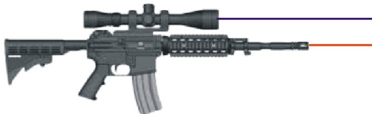
Fig. 1. Classical concept of boresight
