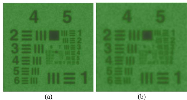
Fig. 7. Magnified image of USAF 1951 resolution target generated by two tubes of different resolution: (a) tube of resolution 64 lp/mm and (b) tube of resolution 40.3 lp/mm (case of high input illumination).
