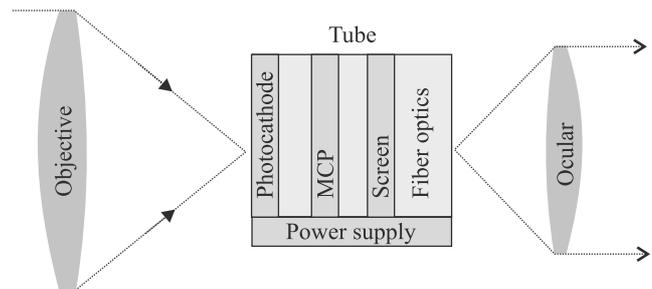
Fig. 1. Block diagram of night vision monocular.
