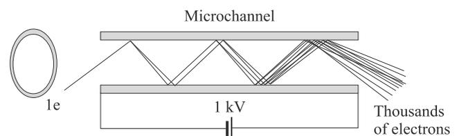
Fig. 11. Principle of work of a microchannel plate.
