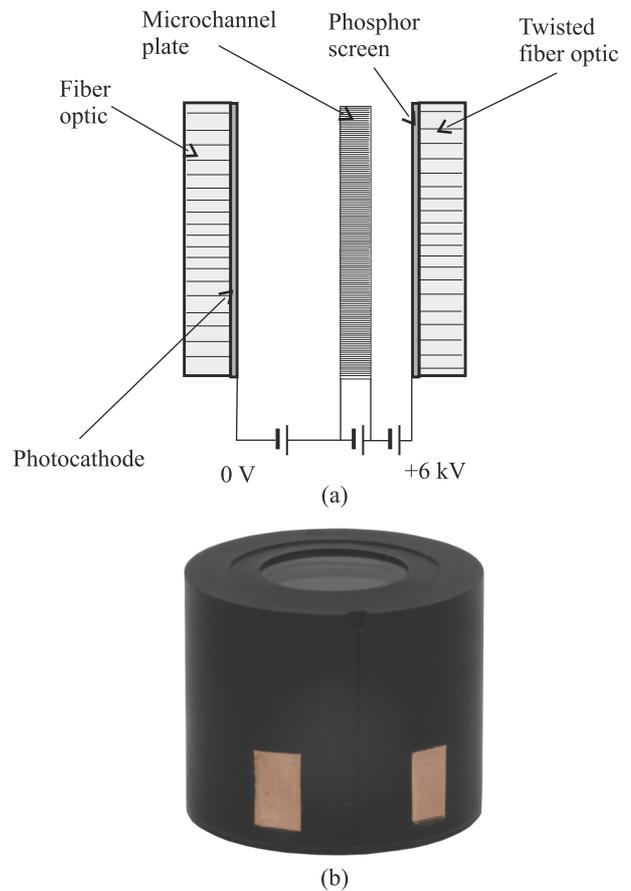
Fig. 13. Proximity focused Gen 2 tube: (a) tube diagram and (b) photo (tube size  $\Phi 35.5 \times 31$  mm).
