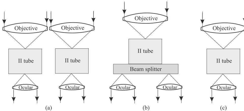
Fig. 6. Block diagrams of three types of night vision devices: (a) bino channel NVDs, (b) mixed-channel NVDs, and (c) mono channel NVDs.
