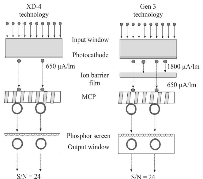
Fig. 15. Two tubes (Gen 2+ tube – XD-4 class and Gen 3 tube) of much different luminous sensitivity generating output image of the same signal to noise ratio (after Ref. 13).
